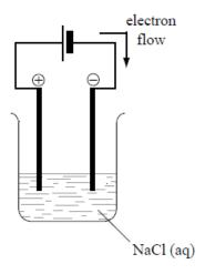
battery/source of electricity connected to two electrodes in the solution with positive and negative electrodes correctly labelled;
